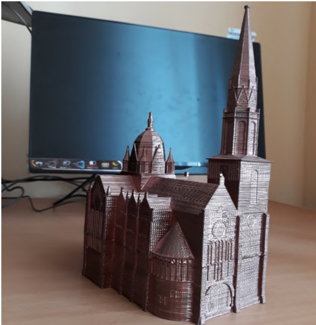
Figure 5: The printed miniature of the Parochial Cathedral of St Mary of Perpetual Assistance.
